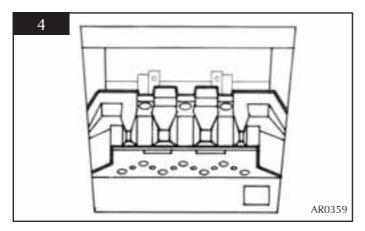
6.2 Locate the rear panel against the spacer brackets and slide down so that it locates on the ledge of the flame baffle, see diagram 5.
